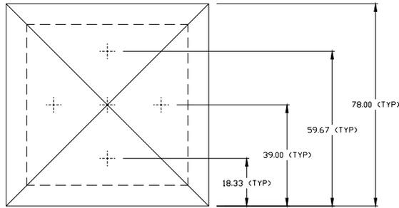
**Figure 9: Accelerometer Locations (Note: all dimensions in inches)**
