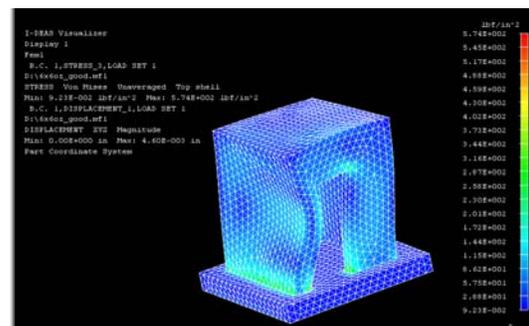
**Figure 4: 5.5 psi load applied to the wall**
