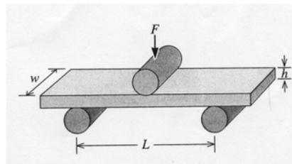
**Figure 2: 3-Point Bending Setup**
