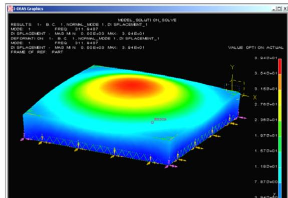
Figure 8: Frequency of the first mode shape
