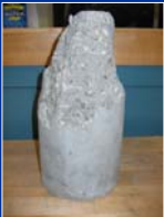
Failed compression specimen
